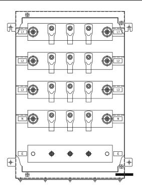
The example is 3-way plus Neutral, with three conductors connected per way.
